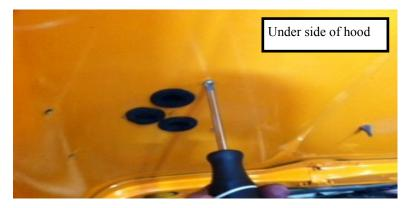
15. Starting with the 3/16" long bolts, secure the Daystar hood vent to the hood.
