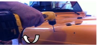
9. Change over to the 1-1/4" hole saw and cut out the three (3) vent holes.
