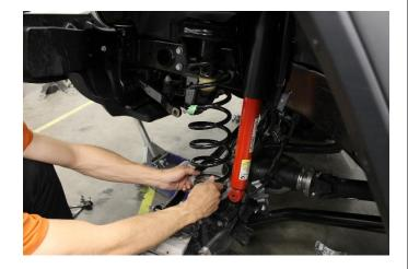
Install Daystar top coil spring Spacer
