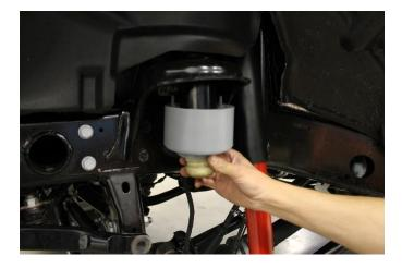
9. Reinstall factory coil springa. Note factory line up on factory lower coil spring isolator
