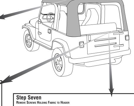
Flip the top fabric back over into the rear of the vehicle (so that the fabric lays backing side up) to expose the plastic strip along the edge of the fabric. Remove the fourteen screws that secure the fabric to the header, setting the screws aside for use in installing the new top. Then remove the old top fabric from the vehicle.
