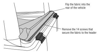
**Manufacturing Note:** Due to a recent header assembly modification by Daimler Chrysler, the plastic strip on the windshield header may have 8 screw locations instead of 14. Both attachment numbers of screws will securely fasten the header and perform as the original design was intended.
