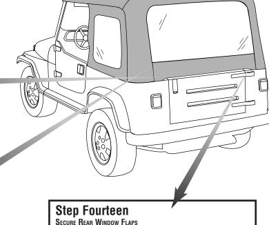
Inside the top locate the flaps sewn to the top on each side of the rear window opening. Pull the flaps over to cover the zipper and tuck them in.
