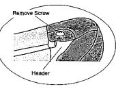
Manufacturing Note: Due to a recent header assembly modification by Daimler Chrysler, the plastic strip on the windshield header may have 8 screw locations instead of 14. Both attachment numbers of screws will securely fasten the header and perform as the original design was intended.
