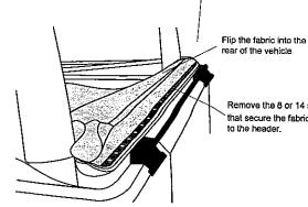
Remove the 8 or 14 screws that secure the fabric to the header.
